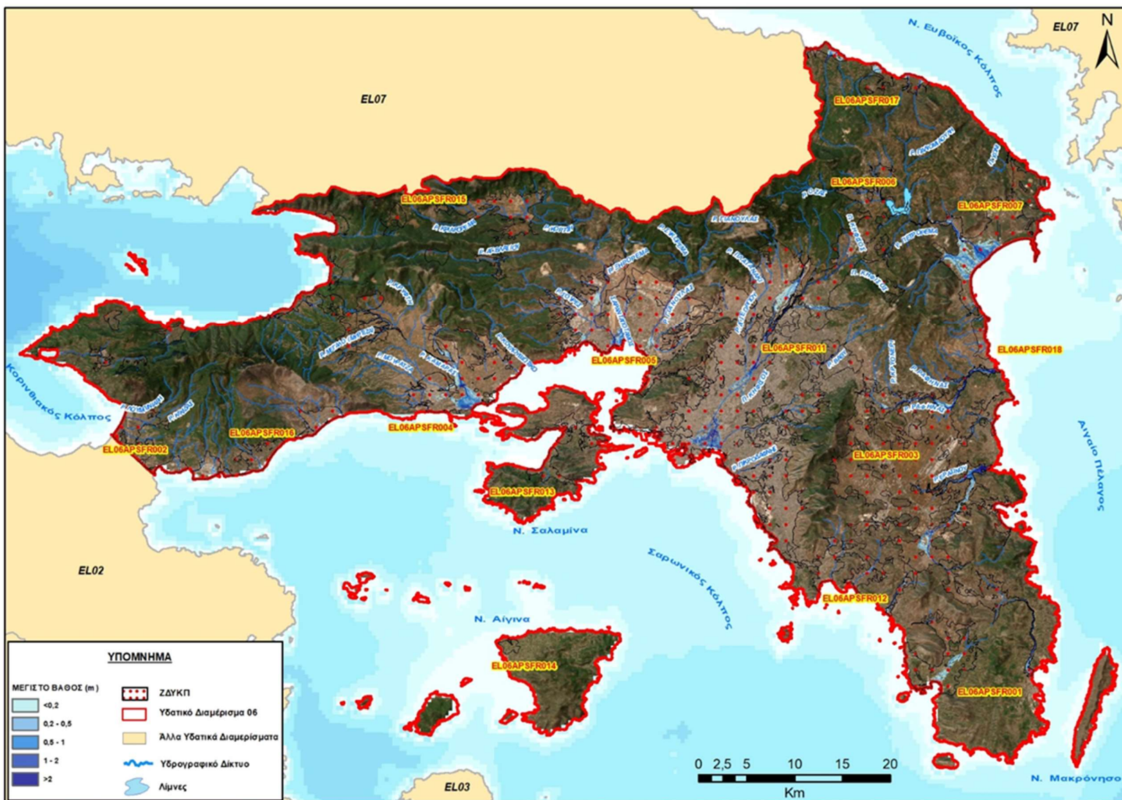
Figure 4-1: Flood areas and flow depths of the River Basin District of Attica (T=50 years)
