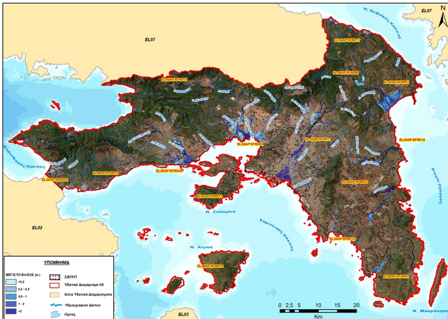
Figure 4-3: Flood areas and flow depths of the River Basin District of Attica (T=1000 years)
