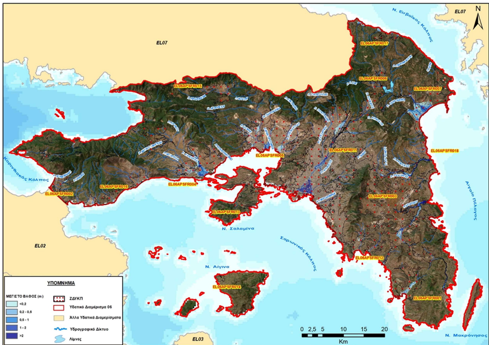
Figure 4-2: Flood areas and flow depths of the River Basin District of Attica (T=100 years)
