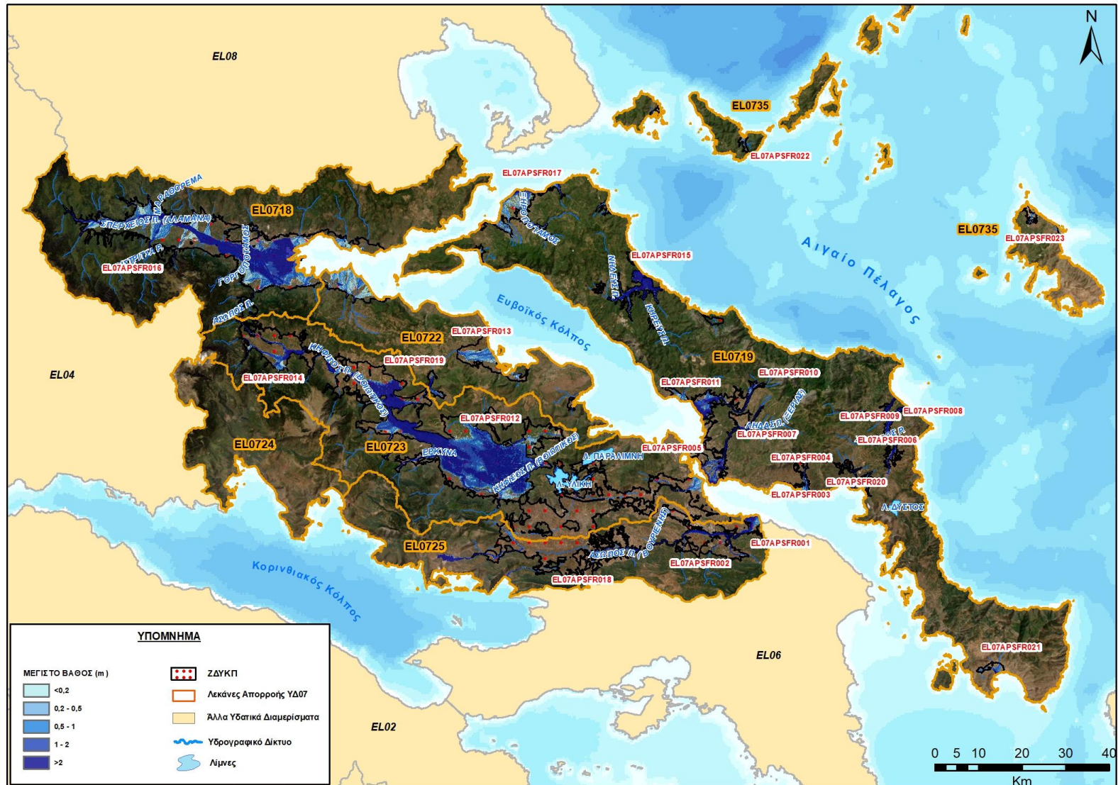
Figure 4-3: Flood areas and flow depths of the River Basin District of Eastern Central Greece (T=1000 years)
