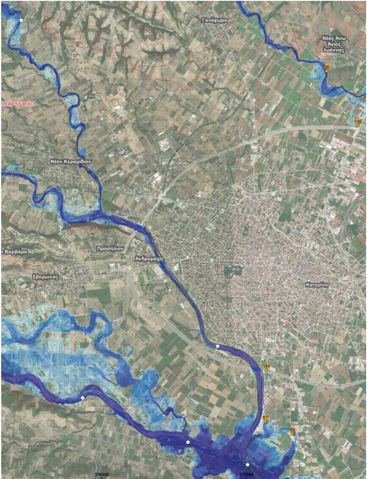
Image 6-1: Part of a FHM showing Katerini area, APSFR EL09APSFR001 with colour gradation of maximum floodwater depths.
