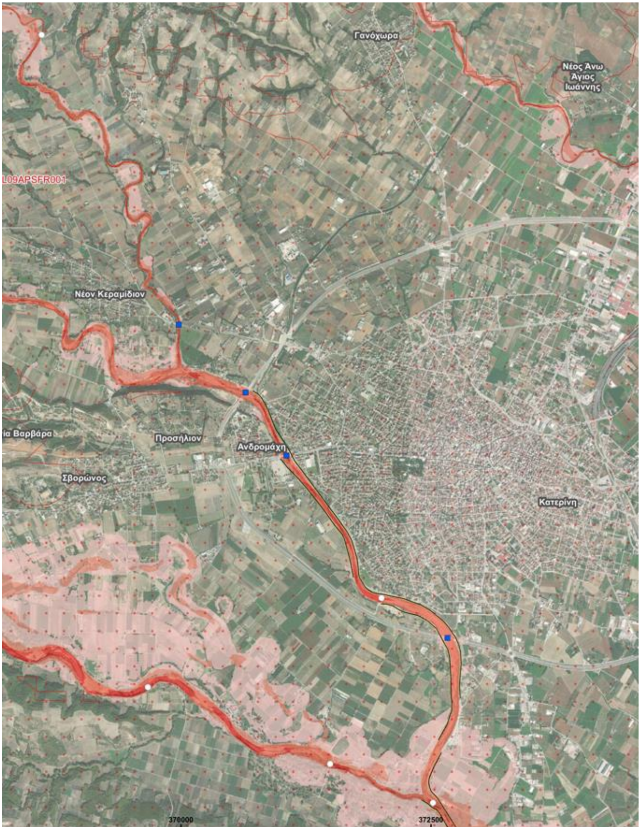
Image 6-2: Part of a FHM showing Katerini area, APSFR EL09APSF001 with colour gradation of maximum floodwater velocities.
