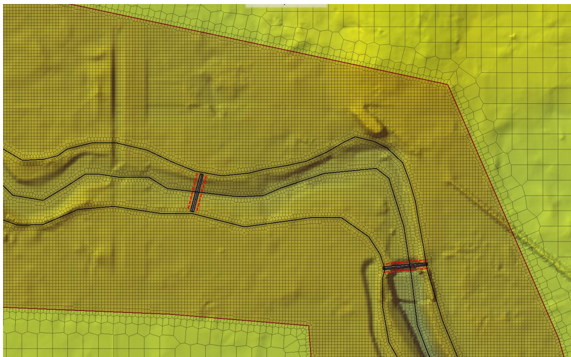
Figure 5-1: Snapshot of the HEC - RAS 6.4.1 graphical environment showing the DTM, the 2D grid and structures perpendicular to the stream flow
