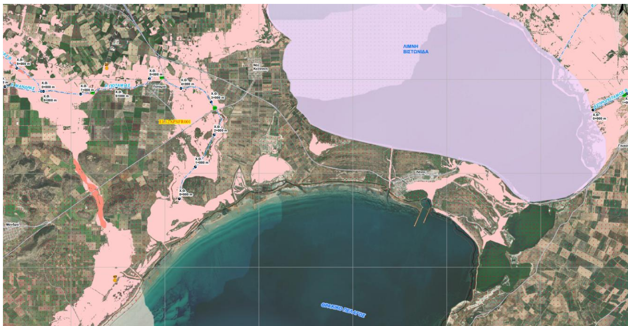
Figure 6.6: Part of FHM (Nea Kessani area), APSFR EL12APSFR001 with colour-coding of maximum floodwater velocities, for T=100 years.
