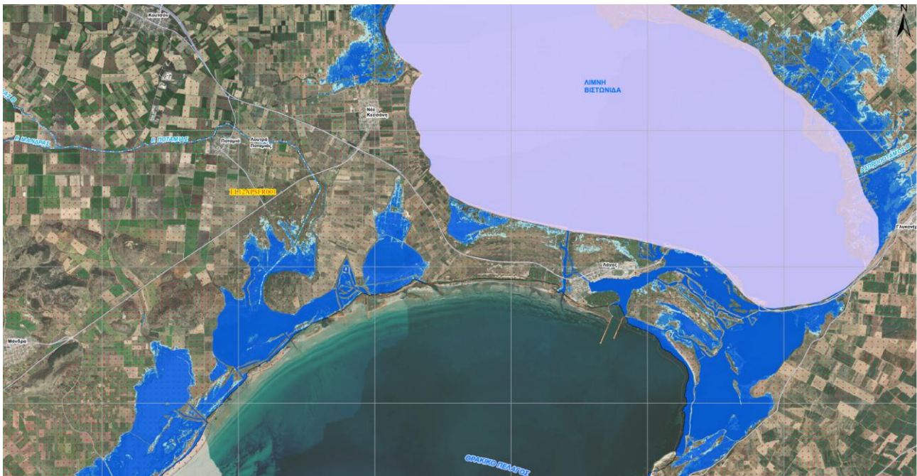
Figure 6.7: Part of FHM from mean sea level rise (Nea Kessani area), APSFR EL12APSFR001 with colour-coding of maximum floodwater depths, for T=100 years.
